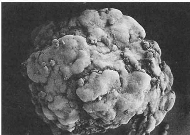
Figure 16. SEM photo showing the adhesion of fine particles on the surface of coarse particle for the PE-CPE system.
